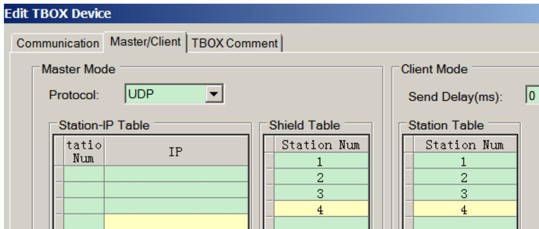
The settings of T-BOX1 and T-BOX2 in the Master mode are shown as following: (turn off DIP switch 1)
