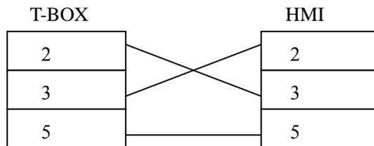
XC series PLC and T-BOX cable connection figure:
