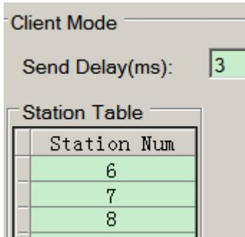
Station number table: station NO.6, NO.7 and NO.8, the purpose is to record the Modbus Slave device station numbers in the T-BOX.
