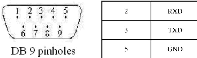
T-BOX and HMI cable connection figure:
