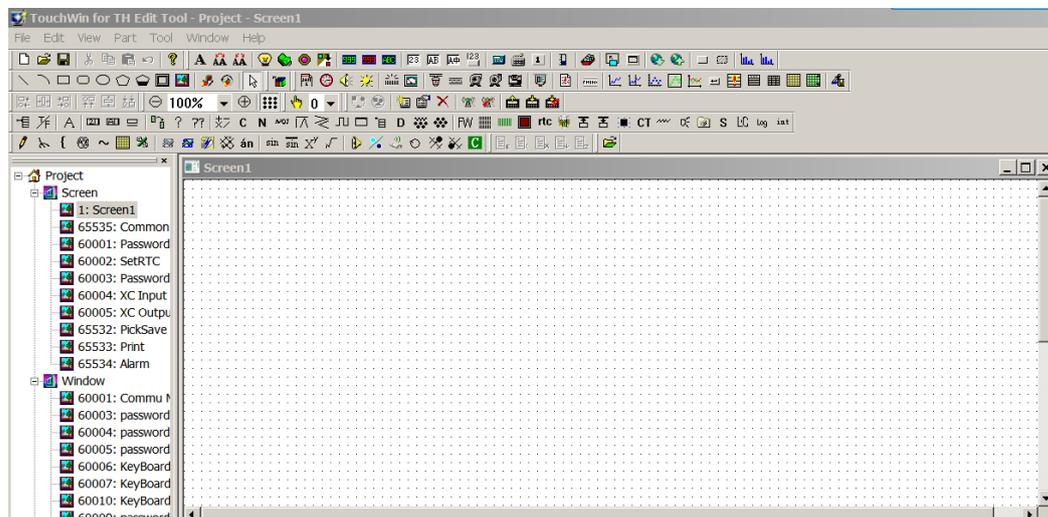
Please note: for all the objects in the project, please change the “PLC port” to network device. For example: the lamp button, change “PLC port” to “thinget XC series”.
