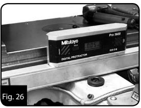
When mounting the reader head if necessary pack the reader head (Fig. 27) so that it travels in line and square to the scale to avoid any damage to the scale. Testing for parallel can be done by either a dial indicator or a precision level. (Fig. 26) The cover must be fitted (Fig. 28)
