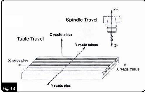
Milling Machine Direction
