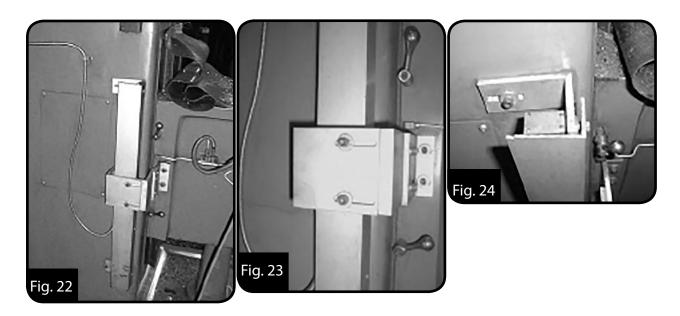
The "Z" axis scale should be installed on the side of the column ensuring that the open side of the scale is away from direct swarf and coolant and that the travel is in the right direction "-" towards the spindle and "+" away from the spindle. The bracket (Fig. 22) is mounted off the knee, and around the scale (Fig 23) to allow for the cover (Fig.24) to protect the scale, where excessive coolant & swarf are present.
