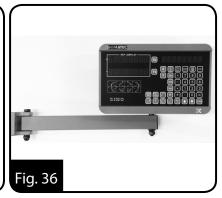
The DRO is mounted to the bracket using the two angle brackets and the mounting pin and secured with the bolt supplied. (Fig. 37)
