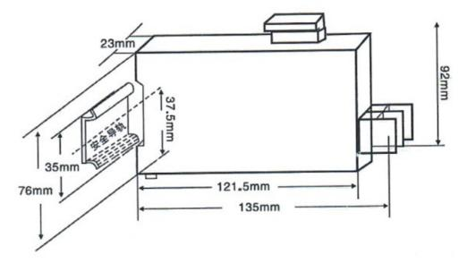
Installation Method: Can be fixed and installed on 35mm standard guide rail
