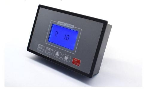
Set the lower limit of speed Press the MENU button 4 times to enter the function 3 key surface Press the plus and minus keys to set Press RUN/STOP to save and exit
