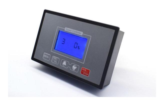
Speed limit setting Press the MENU button 5 times to enter the function 4 key surface Press the plus and minus keys to set the size value Press RUN/STOP to save and exit.
