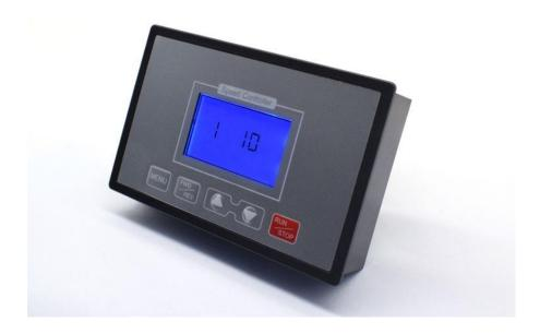
Slow stop time setting Press the MENU button 3 times to enter the function 2 setting key surface Press the plus and minus keys to set the time Press RUN/STOP to save and exit (10 is 1 second, 100 is 10 seconds)
