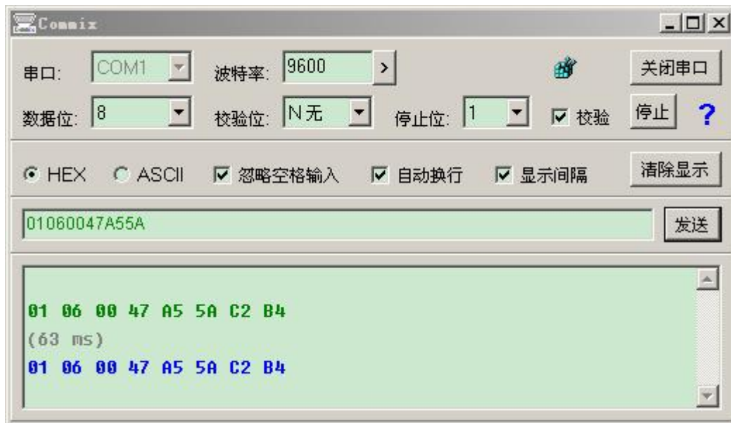
Figure 4-1 Total Zeroing Frame Structure
